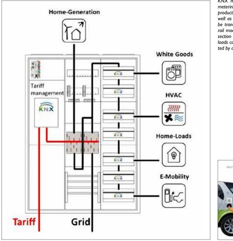
KNX main power distribution board including a metering and a distribution section. The current production of an energy generation system, as well as the consumption of the building itself, can be transmitted on KNX via the meter. KNX DIN rail modules can regulate loads in the distribution section depending on meter values. Moreover, the loads can be adapted to a tariff that was transmitted by an energy manager.
