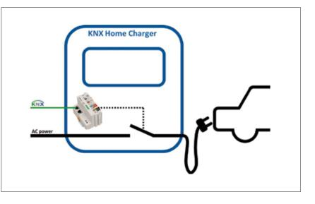
roller and, on the other hand, to enable remote starting of the charging process (closure of the charging contactor).
